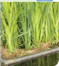
loating reed beds consist of a buoyant tubular framework of welded UV protected polyethylene, supporting a coir mattress, sandwiched between two layers of plastic mesh into which the reeds are planted. Constructed in 4m² units, the floating reed beds are modular in design and can be created in a variety of permutations to meet any area size or shape requirement. They can be installed on sludge lagoons, storm
